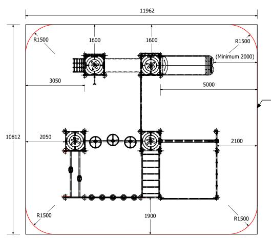
Fallzone at absolute minimum, recommend allowing an extra 100mm where possible from all hard surfaces, including border capping and surround posts etc.
