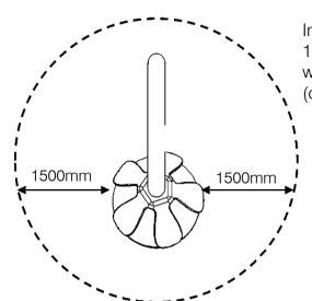
Install instrument with 1500mm free space (from widest point) around it. (drawing not to scale)
