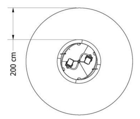
External dimensions of the device: diameter 2640 mm Height of the device from the ground level: 1013 mm Weight of the device: 520 kg
